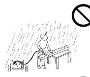
Never operate the generator in wet conditions such as in rain or snow.
