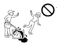
Take care not to spill any fuel on the engine or muffler when refueling.
